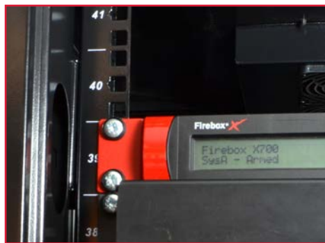
Incremental U-height markings on profiles
